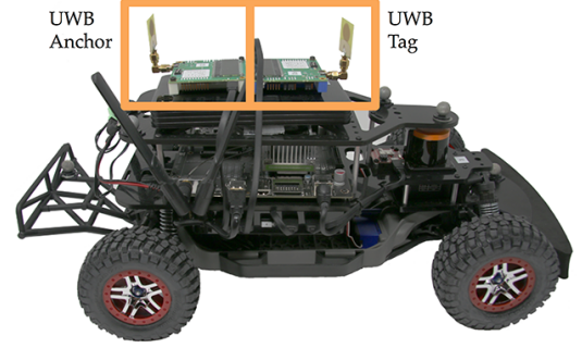
Fig. 3: Two Decawave ultra-wideband radios serve as the range sensors for our system.
